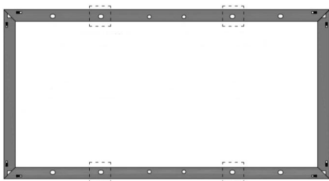
Figure 1.2 : Bolt mounting (4 mounting holes)
